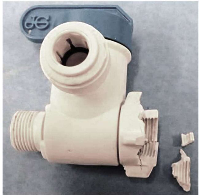
FAILED "ANGLE STOP VALVE PASVPP2", 3/8", FROM "JOHN GUEST ® ".
