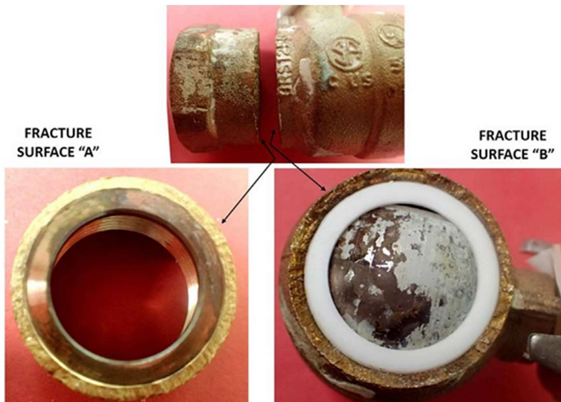
Failure of a brass valve
