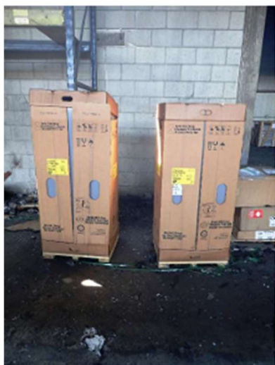
Carboard boxes containing furnaces. Photographs taken after a fire. The boxes show soot.
