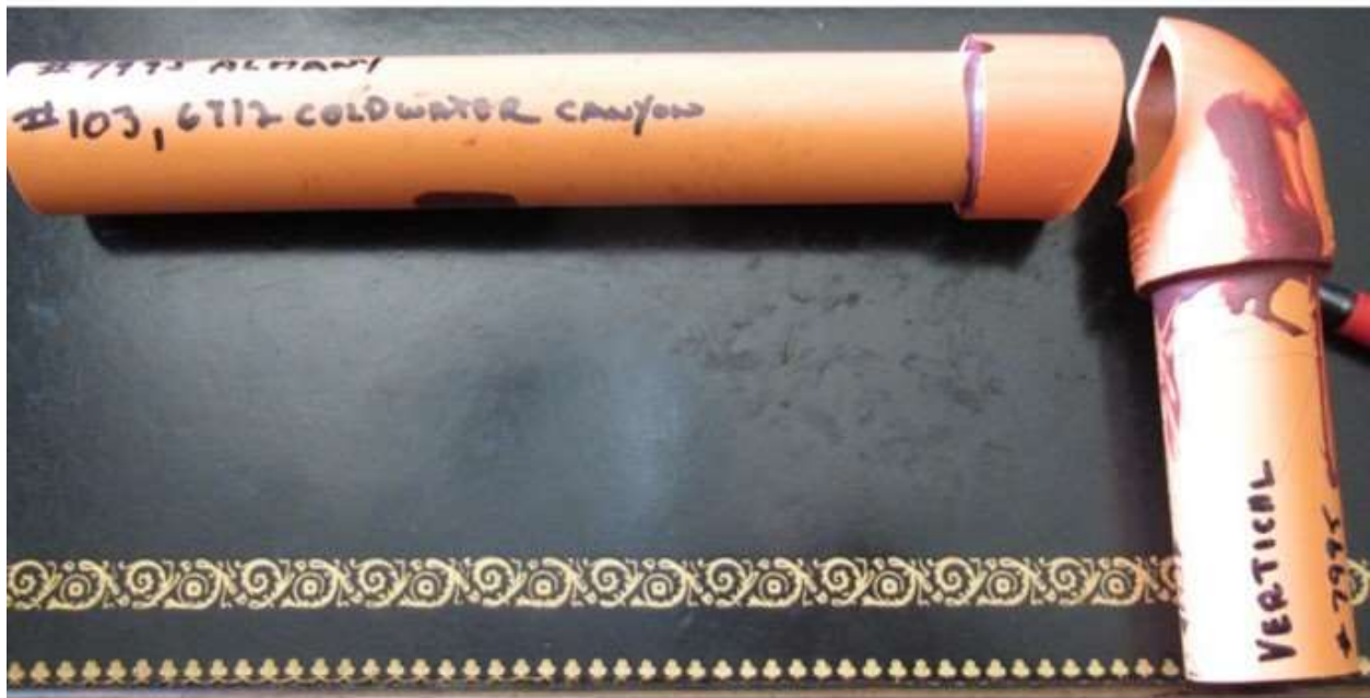
FAILURE OF A CPVC 90-DEGREE ELBOW
